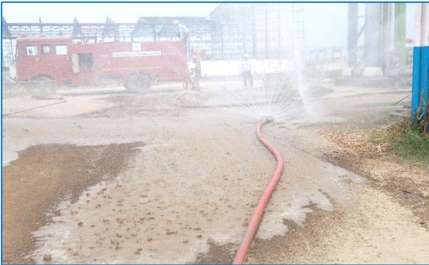
Water curtain at incident spot
